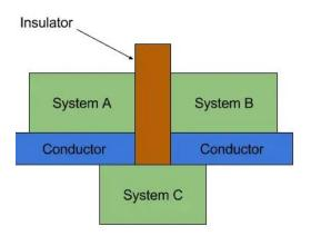
Consider two systems A and B, separated by a wall which does not allow any exchange of energy between them. Such a wall is known as insulating wall or adiabatic wall. The third system C is separated from the systems A and B by a conducting wall.
